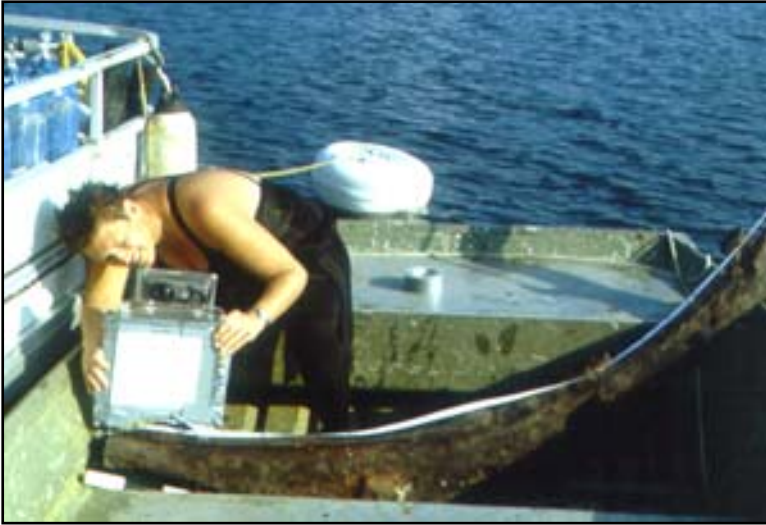
Figure 2: Sue Vezeau uses goniometer to record curvatures of loose timbers from the wreck (SCIAA photo).
